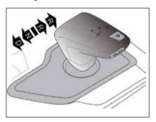
Push or pull the shift lever briefly in the desired direction (two positions forward and backward). When the shift lever is released, it will return to the neutral position.
