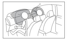
Schematic Diagram for Deployment Area of Side Airbags and Curtain Airbags
