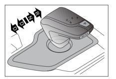
In the automatic mode D gear, move the shift lever to backward to switch to M gear and select the manual mode. To return to D (Drive) gear, move the shift lever to backward D gear.
