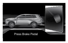
The ACC can use about 40% of the braking capacity of the foot brake, if the front vehicle suddenly brakes on the motorway, the ACC cannot decelerate the vehicle to a safe speed range, then the instrument cluster will display "Press Brake Pedal", the driver shall take the brake intervention immediately.
