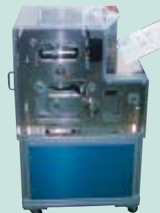
Equipment for completely erasing e-blue™ images (prototype)*
